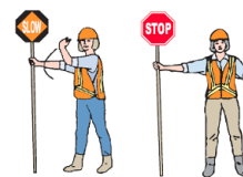
A flagger may direct traffic in a work zone. You must do as the flagger directs.
